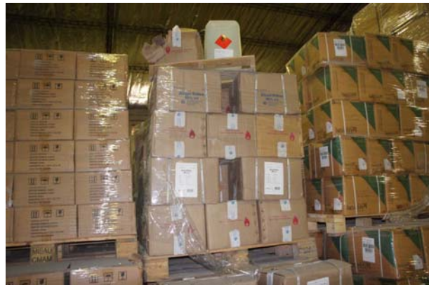
Inflammable commodities stored mixed with other inventory in the Adil warehouse
